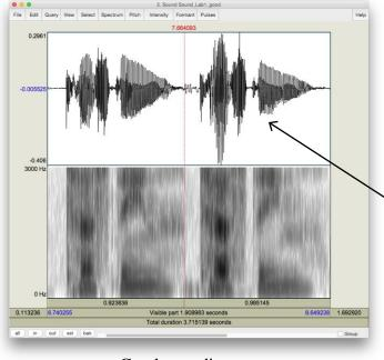
Compare the waveform in these two cases. The one in the clipped recording has a square-like form.
