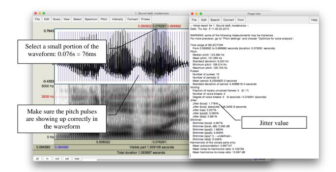
Figure 8.2 Jitter measurement
