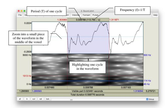
Figure 4.2 Calculating pitch by waveform
