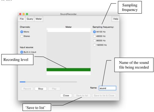
Figure 1.3 Recording a mono sound
