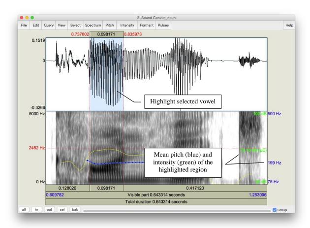
Figure 9.1 Measuring mean pitch and intensity in Praat
